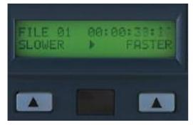
You can increase the speed of the replay of your DV file by pressing the Soft Key under the word FASTER (on the LCD) during **PLAY FORWARD** or **PLAY REVERSE**. Each time you press the Soft Key the speed of replay is doubled, up to a maximum of 32X the original speed of your DV.
